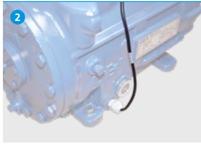
Oil sump heater
